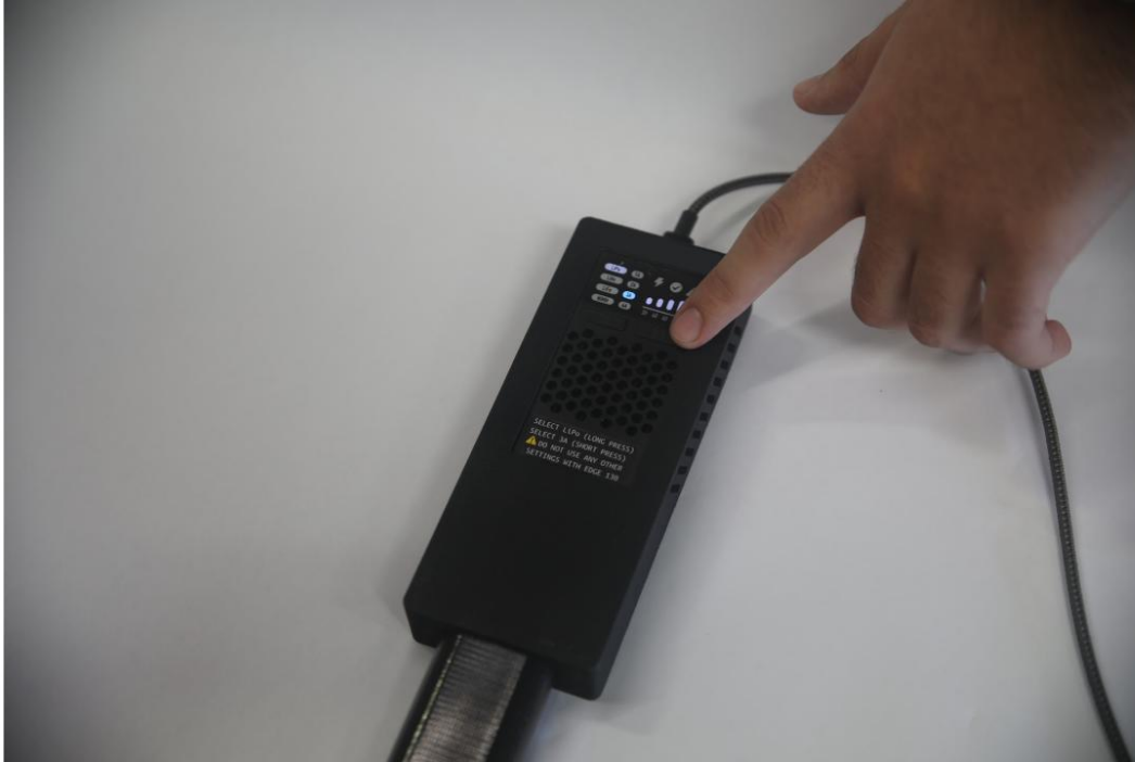
Figure 37 – Initiate Battery Charging
