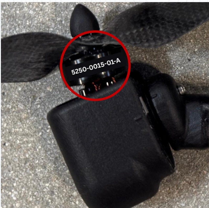
Figure 1 — Motor Part Number “-015” (Old Motor Design)
