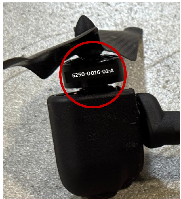
Figure 2 — Motor Part Number “-016” (New Motor Design)
